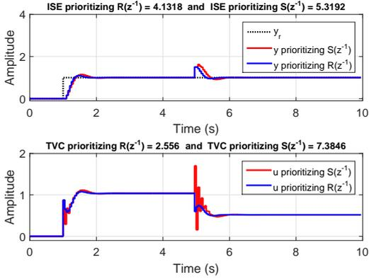
Figure 3: Step response with output disturbance.
