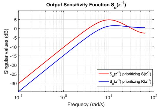
Figure 6: Output sensitivity function.
