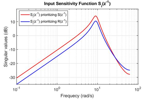
Figure 5: Input sensitivity function.
