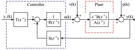
Figure 1: RST digital controller canonical form.
