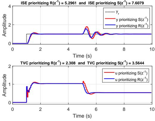
Figure 2: Step response with input disturbance.
