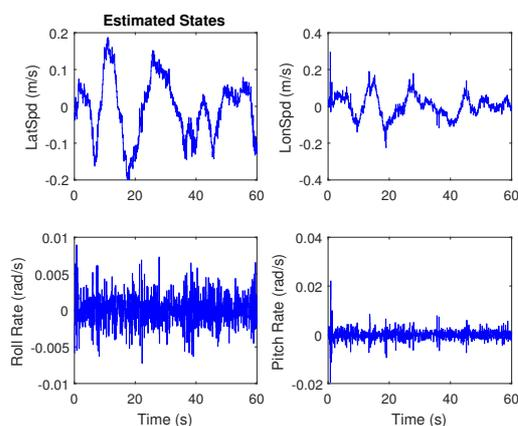
Figure 7: AR.Drone with LQG in real flight: estimated states.
