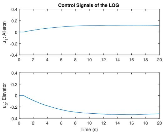
Figure 3: AR.Drone with LQG in simulation: control signals.
