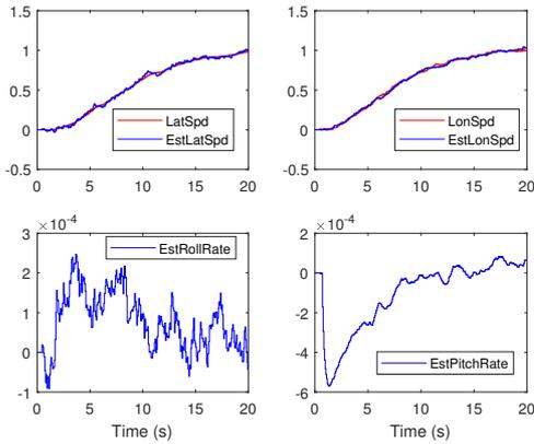
Figure 4: AR.Drone with LQG in simulation: estimated states.
