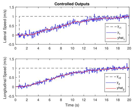
Figure 2: AR.Drone with LQG in simulation: controlled outputs.
