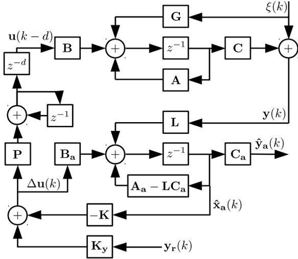
Figure 1: Block diagram of the LQG system.
