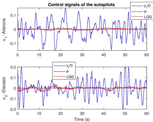
Figure 6: AR.Drone with LQG in real flight: control signals.
