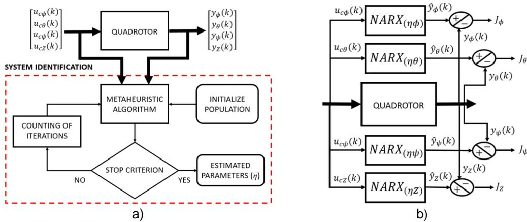
Figure 6 – Structures of quadrotor system identification with metaheuristic: a) General structure; b) Cost functions.
