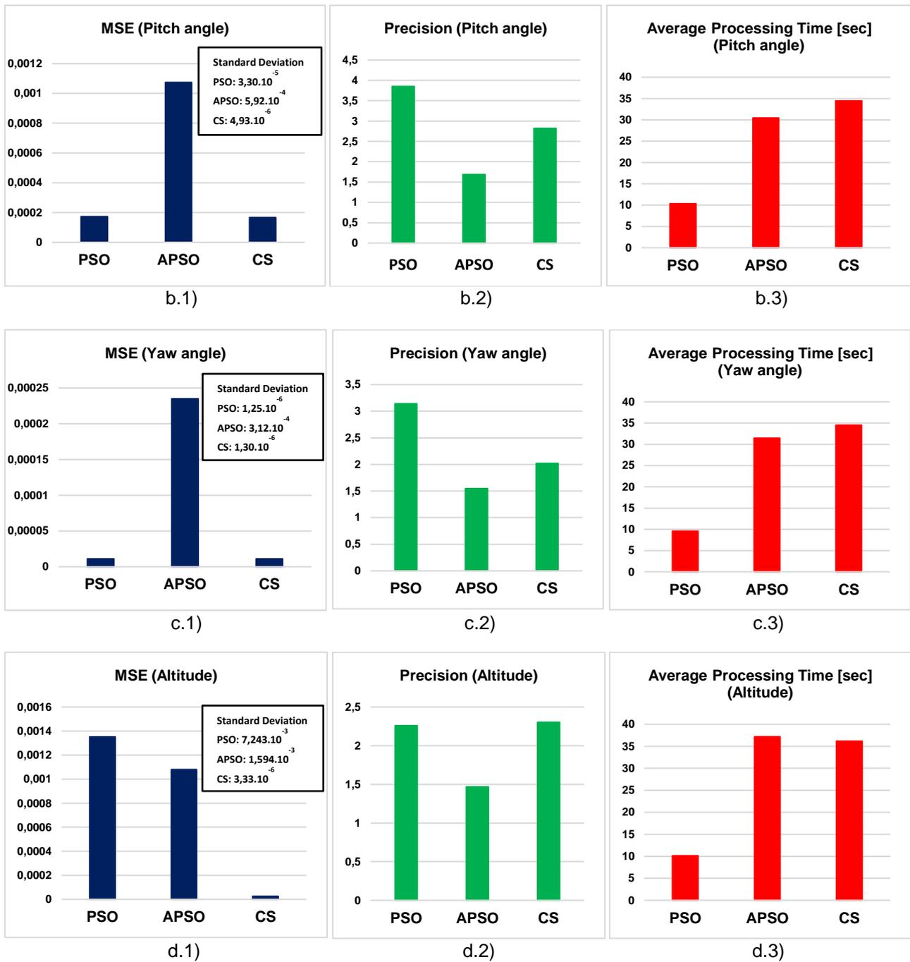
Figure 7 – Results of MSE, precision and APT of metaheuristics in quadrotor system identification: a) Roll angle; b) Pitch angle; c) Yaw angle; d) Altitude.
