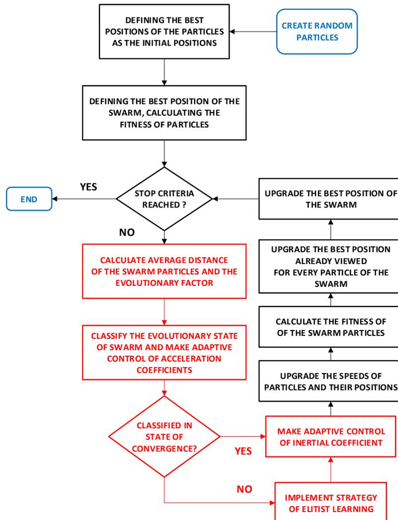
**Figure 3 – Flowchart of APSO algorithm.**
