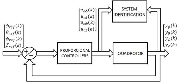
Figure 5 – Block diagram of quadrotor system identification.
