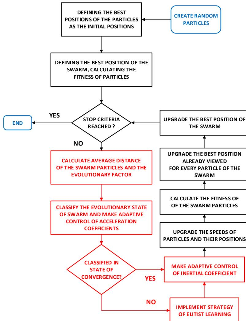
**Figure 3 – Flowchart of APSO algorithm.**
