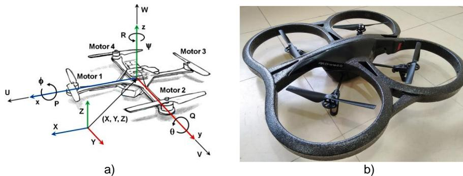
**Figure 1 – Structures of UAV quadrotor: a) Ideal model; b) AR.Drone 2.0.**
