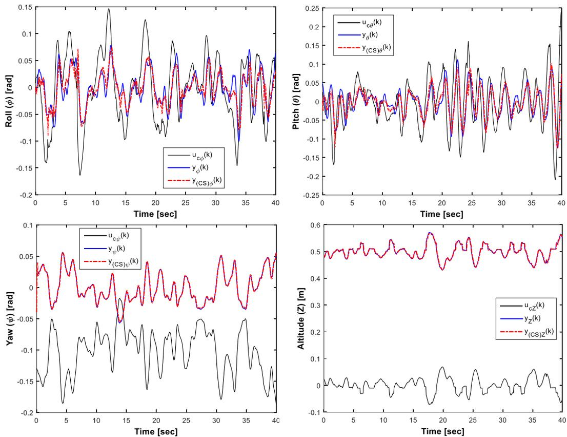
Figure 8 – Original input and output signals, and CS estimated output signals of four state variables.
