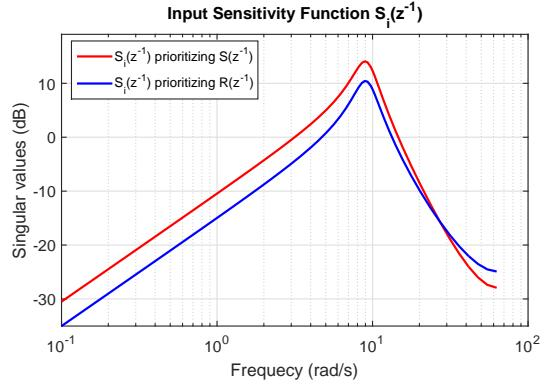
Figure 5: Input sensitivity function.
