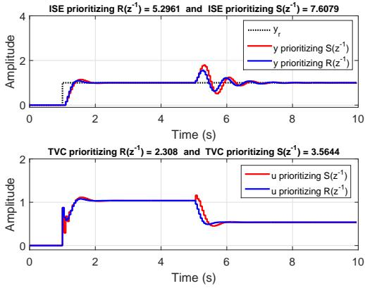
Figure 2: Step response with input disturbance.
