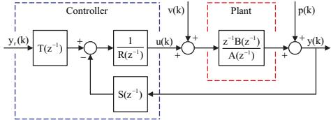
Figure 1: RST digital controller canonical form.
