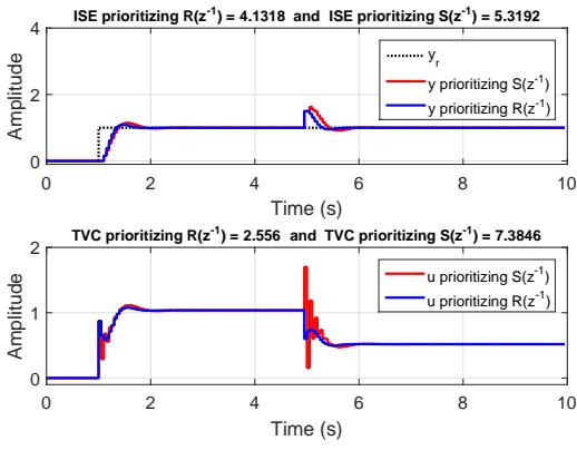
Figure 3: Step response with output disturbance.
